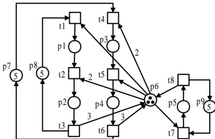
**Figure:** Example for a siphon with only a resource place.
