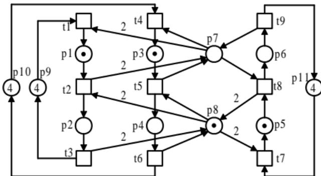
Figure: A live  $S^4R$  net with a  $\max''$ -controlled siphon.
