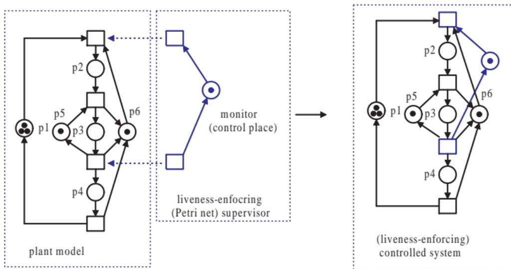
Figure: Plant, supervisor, and controlled system.
