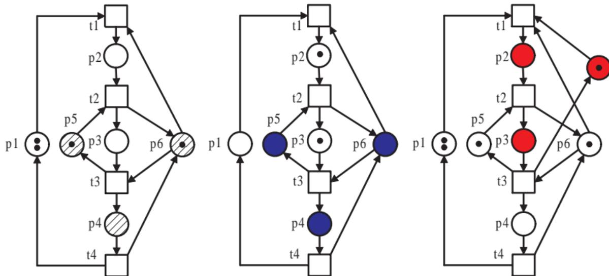
**Figure:** (a) A Petri net, (b) a dead marking, and (c) a controlled siphon.
