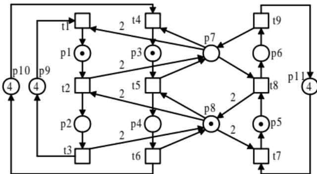
Figure: A live  $S^4R$  net with a non-max'-controlled siphon.
