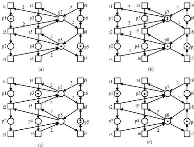
Figure: (a) and (b),  $S$  is max''-marked, and (c) and (d),  $S$  is non-max''-marked at the shown markings.
