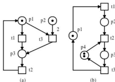
Figure: Two Petri nets, (a) is deadlock-free, (b) is live.
