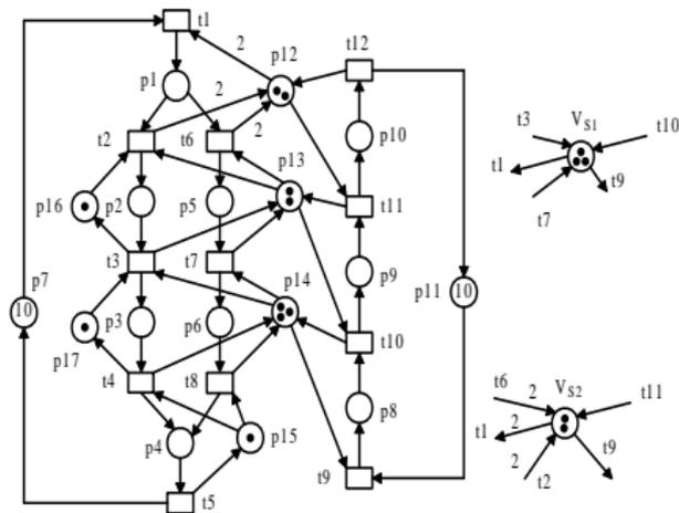
**Figure:** A siphon is max-controlled in a generalized Petri net  $(N_1, M_1)$ .
