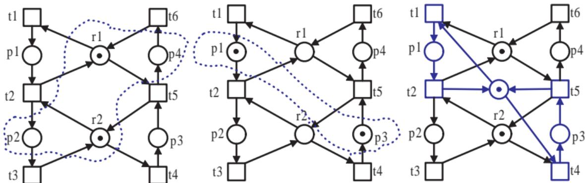
Figure: siphon, token loss, and its control.
